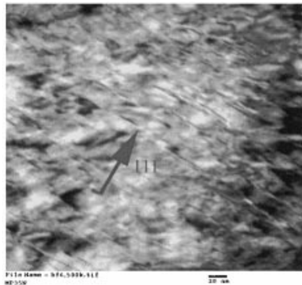
Fig. 3. Transmission electron microscopy image showing fine planar defects formed on \{111\} habit planes in MP35N.
